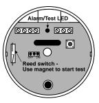
the "T" on the case. Placing a magnet next to the "T" when the unit is in the test mode will terminate the test.
